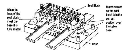
To secure the seal block:
